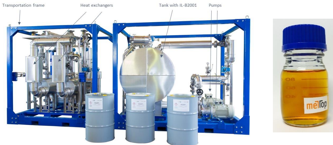
Figure 3: Basic design of an ILTEC system as installed at ArcelorMittal Bremen GmbH in Germany (left) and photo of the optical appearance of the ionic liquid IL-B2001
